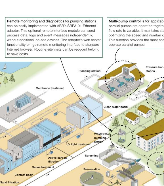
Multi-pump control is for applications where several parallel pumps are operated together and the required flow rate is variable. It maintains stable process conditions optimizing the speed and number of the pumps needed. This function provides the most energy efficient way to Pressure boosting Gas storage tank Sludge drying Humus Gas-fired power plant Catalyst
